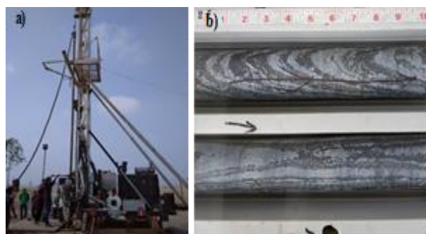
Fig. 4 Photographs showing (a) the LF Core Drill–90 drilling rig and (b) representative basement rock core samples.
