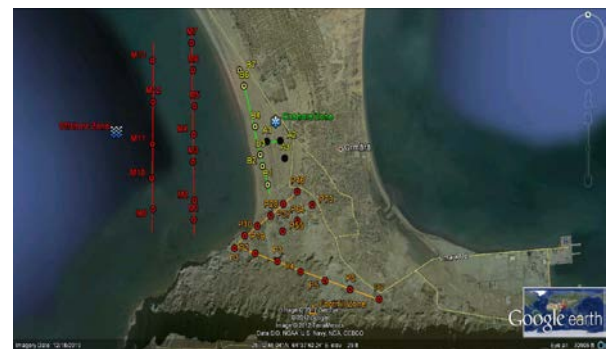
Fig. 4 Site investigation Plan and boreholes location.
