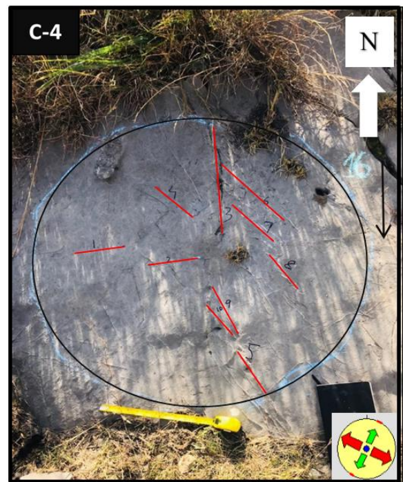
Fig. 6 Circle 4 (C-4) showing medium to high fracture density and joint density is 4.58 \text{ m}^{-1} . The radius of the circle is 45 cm and the area is 6358.5 \text{ cm}^2 ( 0.63 \text{ m}^2 ). Two joint sets are observed.
