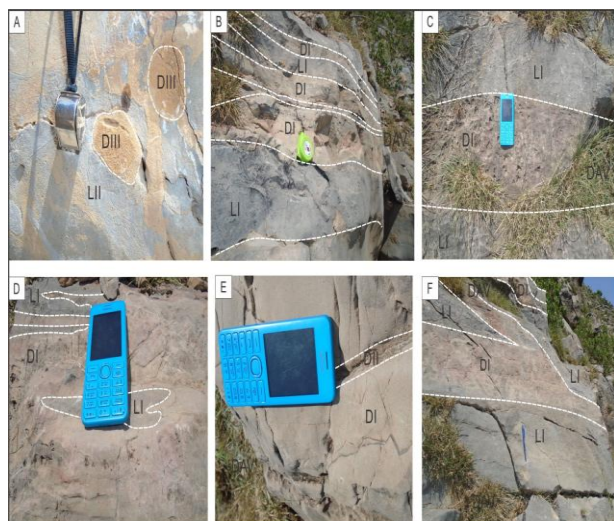
Fig. 8 (A) Shows yellow color augen like dolomites (DIII) in fine grained light grey limestone (LII) facies of Samana Suk Formation at basal part.( B) bedding parallel dolomitic beds light yellowish in color (DI) in dark grey to bluish limestone (LI) facies of Samana Suk Formation at middle part (C) brownish dolomite (DI) in limestone facies. (D): irregular dolomitic effect on limestone facies, light yellowish dolomite (DI), dark grey to bluish limestone (LI), (E) Thick dolomitic bed (DI) is cross cut by dark brown dolomitic vein (DII). (F) Limestone facies (LI) is cross cut by brownish dolomitic beds (DI).
