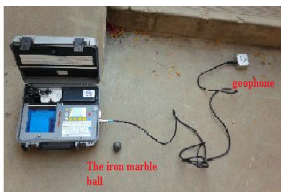
Fig. 3 Vibration device and the steel ball used in the tests.
