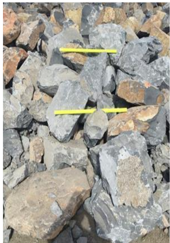
Fig. 8 Oversize piled at a separate stockpile. Scale is 1m.
