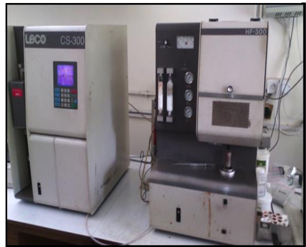
Fig.6 Displaying the CS-300 instrument used for determination of organic carbon content of rock samples procured from the measured section of the Nammal Formation.
