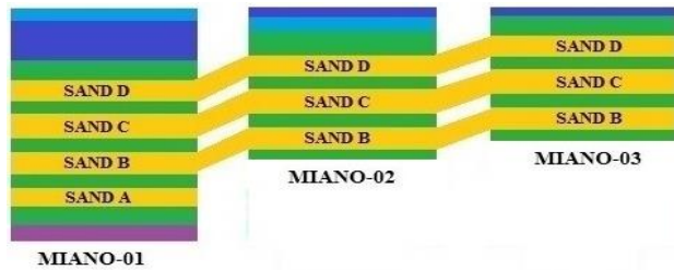
Fig. 6 Intercalation of clay and sand profile in Lower Goru reservoir of Miano wells.
