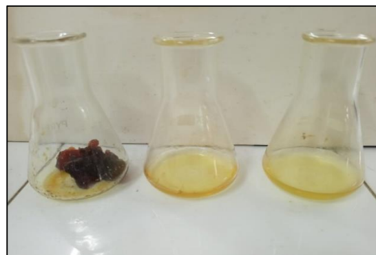
Fig. 2 Showing (L to R): (a) Raw glycerol obtained from biodiesel production, (b) pre-treated glycerol and (c) purified glycerol after bio-adsorbent treatment.
