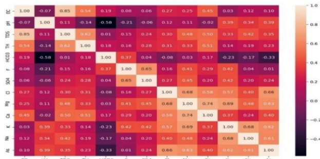
Fig. 4. Correlation matrix of physicochemical parameters (pH, EC, TDS, TH), anions (HCO 3 - , Cl - , SO 4 2- , F - ), cations (Ca 2+ , Mg 2+ , Na + , K + ), and arsenic (As) in groundwater samples.
