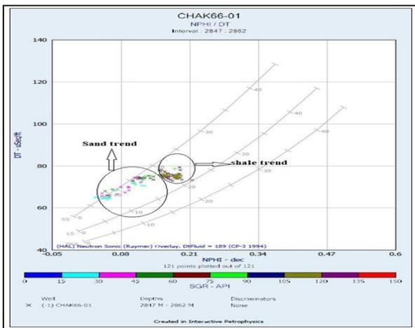
Fig. 8 Cross plot of Nphi and sonic log.
