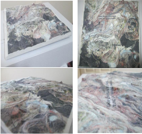
Fig. 10 Colored solid model produced in the 3D printer of the mine site.
