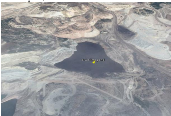
Fig. 7 Slime pond formed in the mined out hole of 6-C panel.
