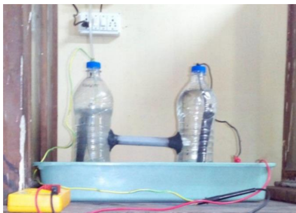
Fig. 1 Microbial Fuel cell for the purpose of water treatment (Prasad et al., 2015).
