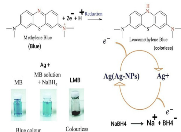
Fig. 4.2 Mechanism of degradation of Methylene blue dye using Ag-PSty-PNiPMaM-MaA-CS catalyst.
