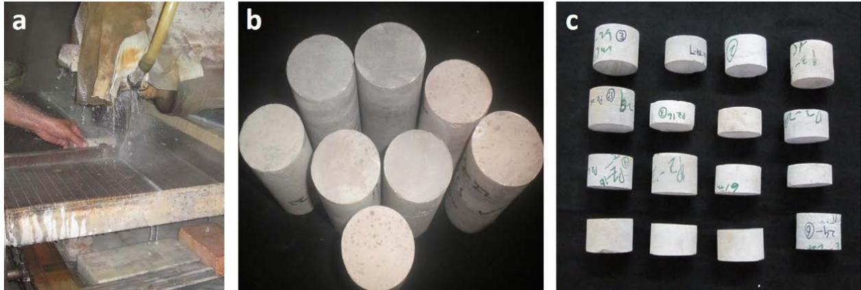
Fig. 3 (a) Cutting of core samples (b) prepared samples for UCS (c) prepared samples for PLT and SRHT.
