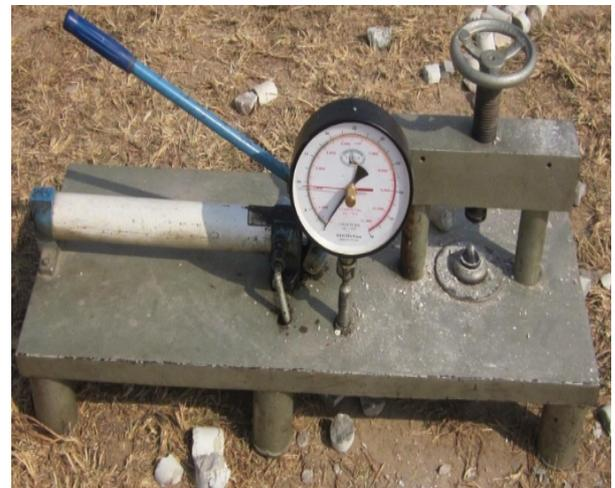
Fig. 5 Point load tester.
