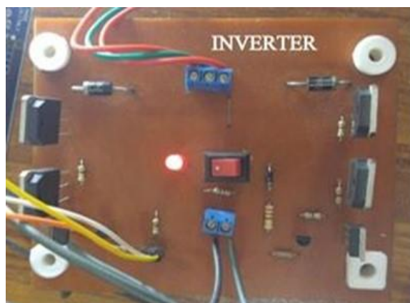
Fig. 1 Grid tie inverter.
