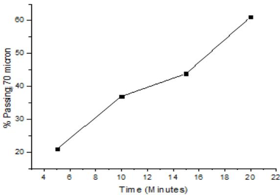
Fig. 4 Effect of grinding time on particle size.
