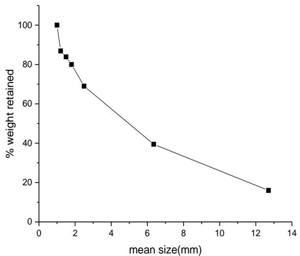
Fig. 3 Particle size curve for roll crusher.
