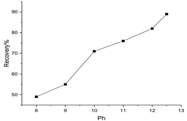
Fig. 6 Recovery of copper as a function pH.
