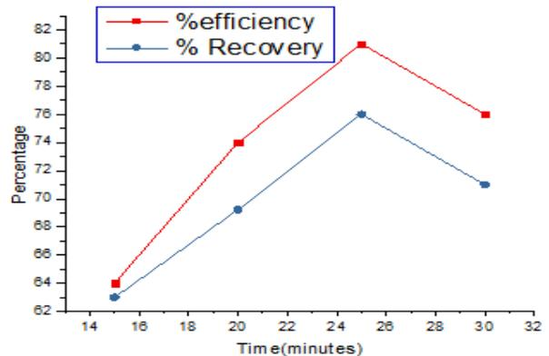
Fig. 7 Recovery of copper as a function of grinding time
