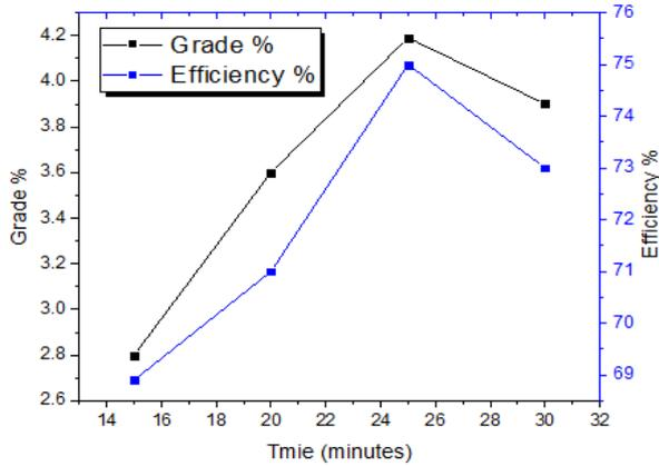
Fig. 8 Effect of grinding time on grade.
