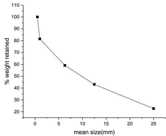
Fig. 2. Particle size curve for jaw crusher
