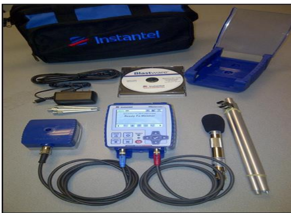
Fig. 2 Instantel micromate vibration measuring device.
