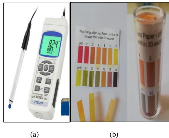
Fig. 2 Laboratory tests using; (a) a pH meter, and (b) a wide range of pH test paper.
