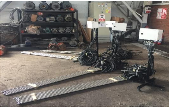
Fig. 3 Temperature measurement probes and data logger
