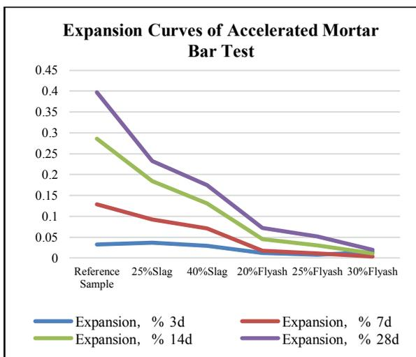
Fig. 6 Expansion of concrete specimen at different ages.
