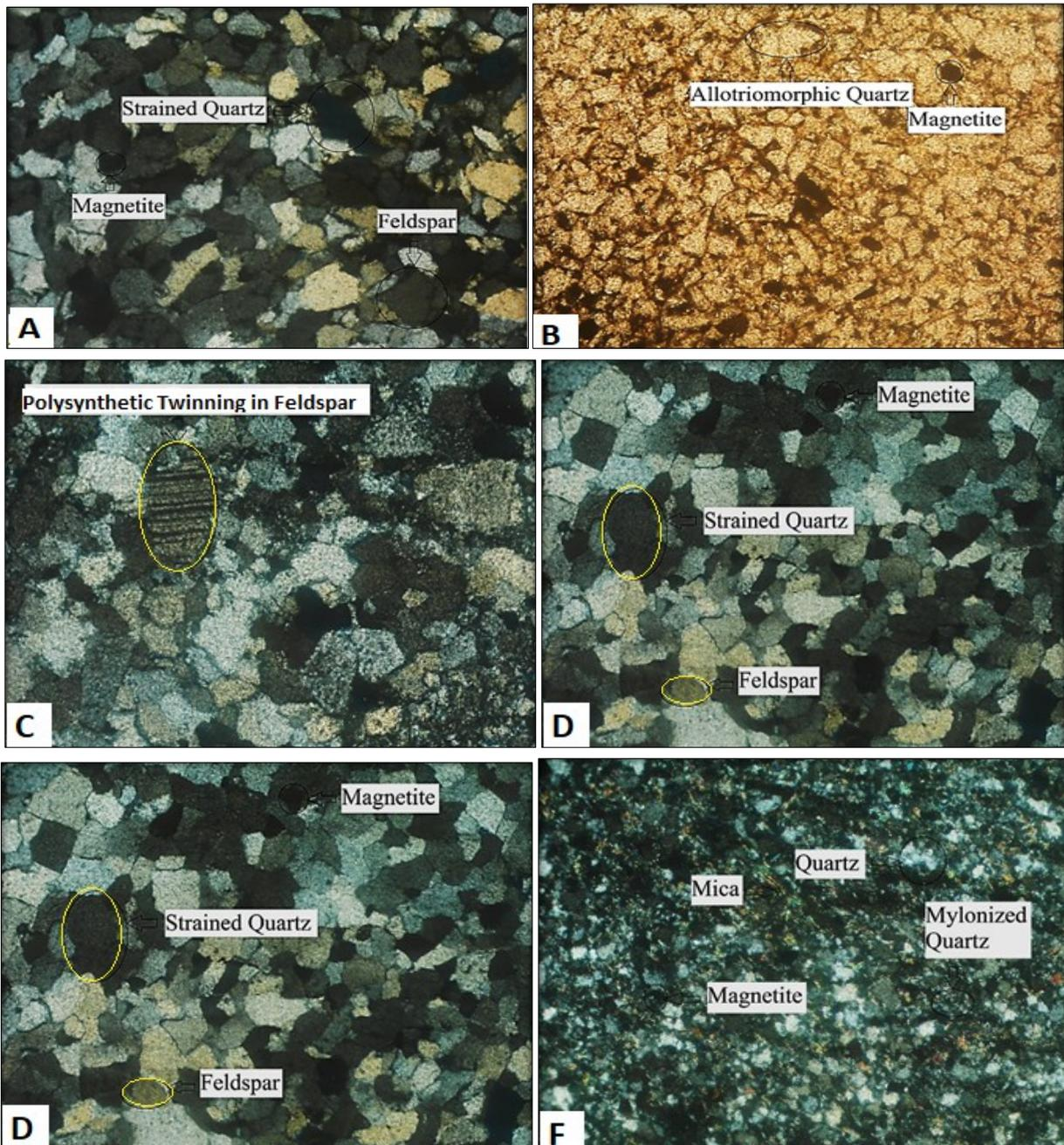
Fig. 4 Microphotograph of river bed aggregate A) strained quartz, magnetite and feldspar, B) allotriomorphic quartz and magnetite, C) polysynthetic twinning in feldspar, D) strained quartz, magnetite and feldspar, E) highly strain quartz, F) mylonized quartz, quartz, magnetite and micas.
