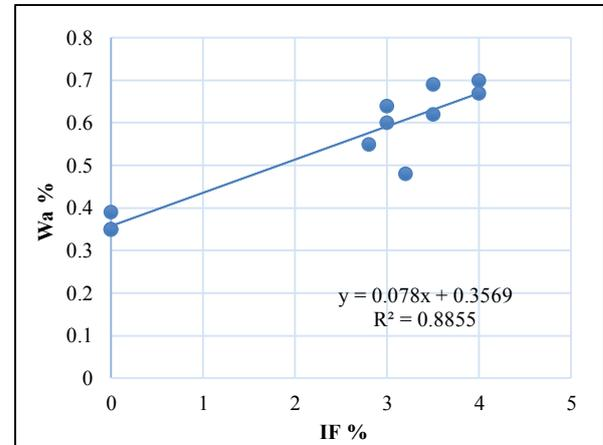
Fig. 2 Correlation between Water Absorption (W<sub>a</sub> %) and Flakiness Index (I<sub>F</sub> %).
