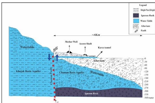
Fig. 3 Sketch showing Karez model, a centuries-old technique to tap water from a source through an excavated tunnel in the alluvium/alluvial fan of mountain foothills. Spaced vertical shafts/wells are dug through the tunnel to remove excavated material and piled up around the shafts / open wells to protect from rainwater to flush in. Mother well is where the water table can be found, and the outlet is the last point where water can be brought to daylight to irrigate land and for domestic use.
